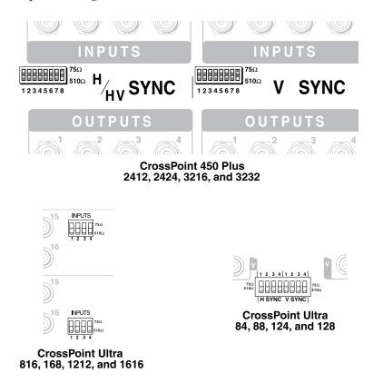
Figure 2-16 — Sync termination switches
